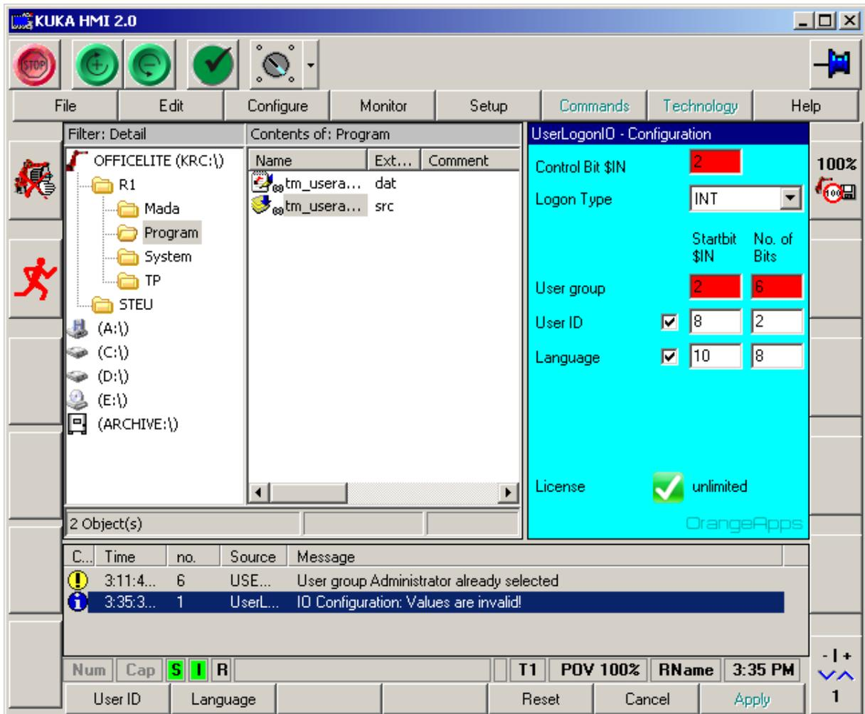
Figure 7-4: error detection configuration KRC2
