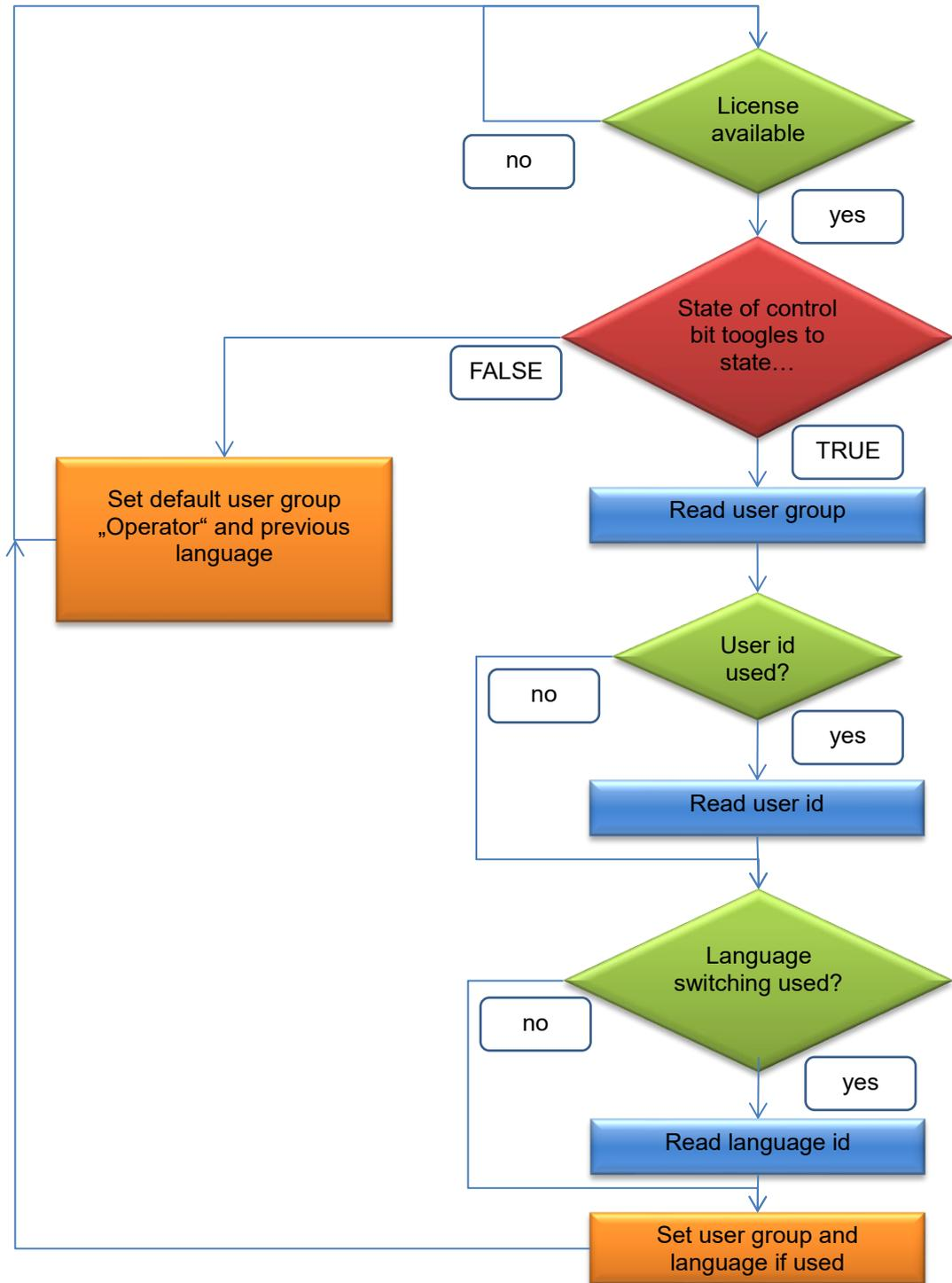
**Figure 6-1: Flowchart Logon to robot system**
