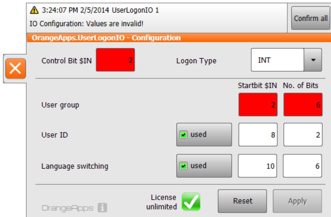
Figure 7-2: configuration error detection plugin KRC2
