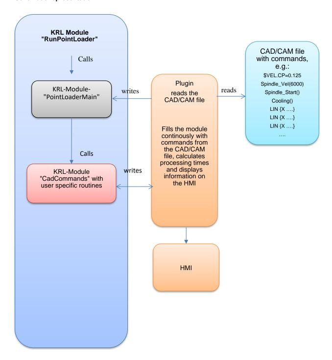
The selection and loading of the CAD/CAM file is done via the HMI buttons. After successful loading, the KRL module "RunPointLoader" is automatically selected. From there, the working program can be started by the operator. In order for the buttons on the HMI to be active, no program may be selected in the robot.
