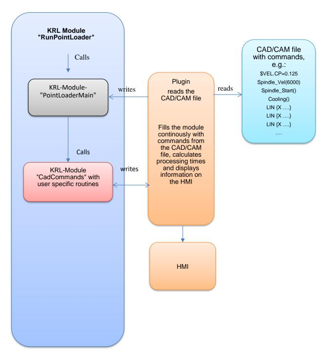
The selection and loading of the CAD / CAM file is done via the HMI buttons. After successful loading, the KRL module "RunPointLoader" is automatically selected. From there, the working program can be started by the operator. In order for the buttons on the HMI to be active, no program may be selected in the robot.
